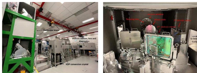
Fig 5 – Left: L4n beam transport and SHG chamber, Right: Dichroic mirror, Beam Diagnostics, Phase Plate beam homogenizer, and focusing lens for L4n beam. The synchronization between L3 and L4n beams has been tested.
