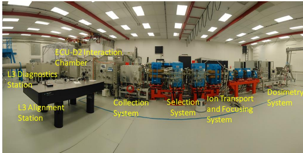
Fig 6 – Photo of the ELIMAIA beamline in E4. The main sections of the ELIMAIA beamline (Ion Accelerator and ELIMED) consist of different subsystems: (i) acceleration, collection and diagnostics; (ii) selection, transport and diagnostics; (iii) dosimetry and sample irradiation.
