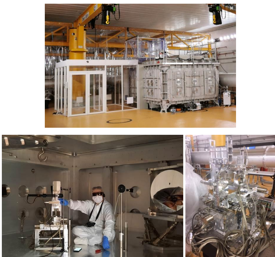
Fig 7 – The ELI-NP E1 experimental area (top), Inside of vacuum chamber (bottom-left), and the completed solid target positioning system (bottom-right).
