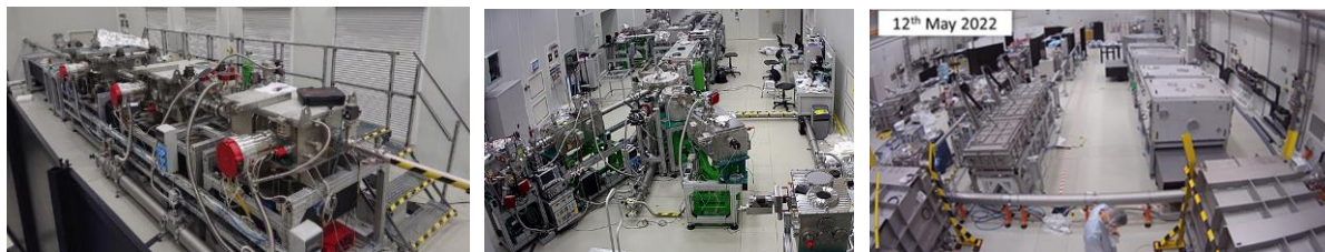
Fig 1 – HR driven 100 kHz gas high-harmonic generation beamline (left), SYLOS driven 1kHz gas high-harmonic generation beamline (centre), SYLOS driven high field interactions: area overview (right).
